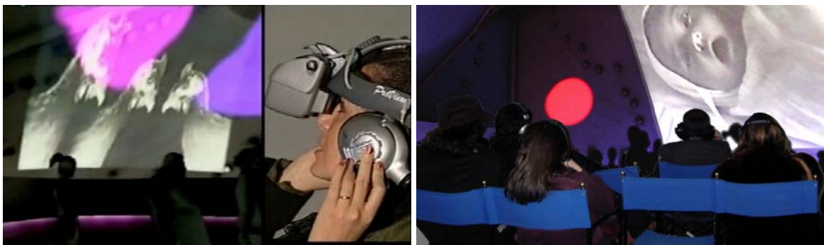
Figure 5. Single user setup with stereoscopic helmet and binaural audio (left); multiple user setup, with monoscopic screen and multichannel audio (right)
